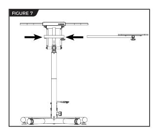
• Unscrew the Adjustment knob and insert the Side Table Assembly into the RIGHT or LEFT end of the Side Table Connector Tube located on the Desktop Post (Figure 7).
